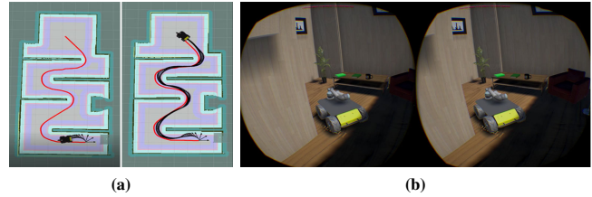
Figure 6: VRGym-ROS bridge. (a) The robot navigation in the scene imported into the Gazebo, exported from the VRGym. The red curve indicates the path planned by the robot’s global planner. The black curve is the actual trajectory executed by the robot. (b) A Husky-UR5 robot is imported into VRGym from ROS to guide the way and open the door for a human agent.
