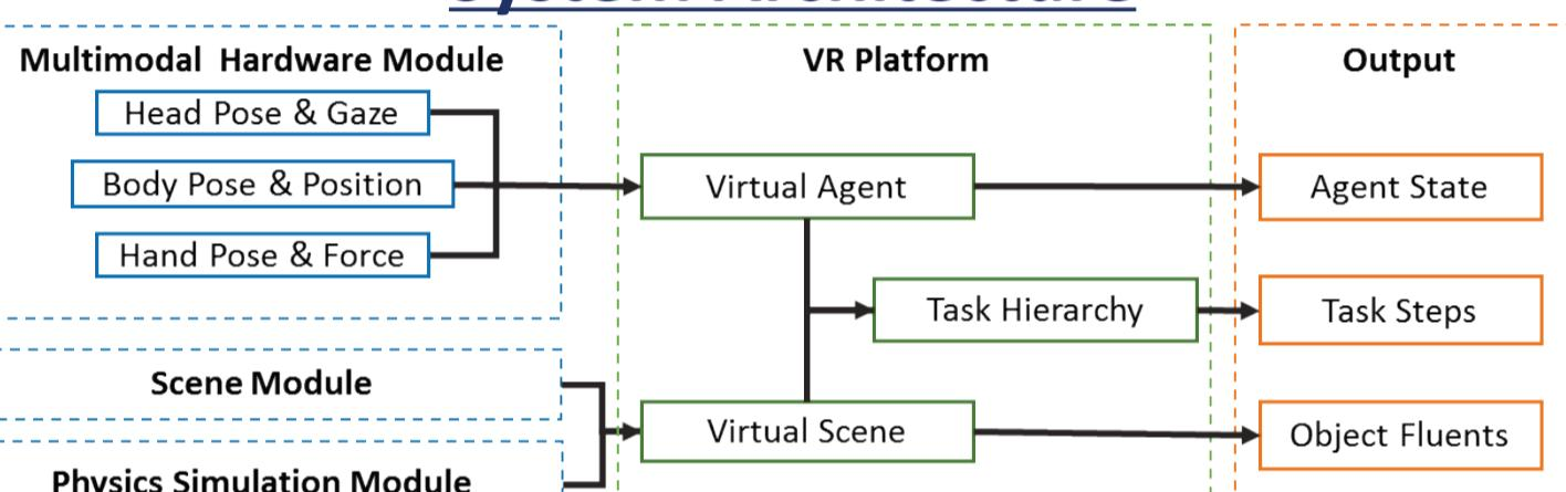
Our system is composed of three sub-modules: i) a Multimodal Hardware, which collects data about the real world agent (*e.g.* head pose, body pose, hand pose), ii) a Scene Module, which provides 3D data about the virtual scene, and iii) a Physics Simulation Module, which simulates the interactions between virtual agent and scenes. These sub-modules are consolidated in our VR platform, allowing the real world agent to interact with the virtual environment.
