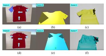
Fig. 4: Six virtual environments with different fidelity for learning and evaluating the knowledge of folding clothes. (a) Grasp areas are recorded. (b) Grasp point is visible and recorded. (c) Full physics-based simulation but with only grasp points recorded. (d) Grasp point is recorded but the trajectory is the pre-defined line. (e) Grasp point is recorded but the trajectory is estimated. (f) Full physics-based simulation with the complete trajectory recorded.
