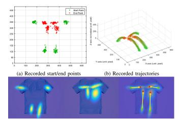
(c) Estimated start points(d) Estimated end points(e) Estimated trajectories Fig. 3: Trajectory analysis using Gaussian fitting. Given a human demonstration of cloth-folding sequences in terms of (a) grasp points and (b) trajectories, our algorithm aggregates the raw data and fits the (c) start points and (d) end points with a Gaussian distribution; (e) folding trajectories are further estimated.
