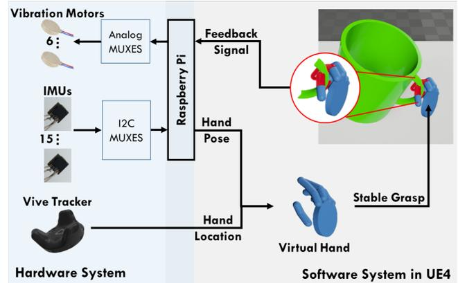
Fig. 2: Schematics of the system architecture. A Vive Tracker and a network of IMUs provide comprehensive hand pose and location in the VR simulator Unreal Engine 4 (UE4). When a stable grasp is formed based on the contact geometry, the virtual object follows the hand’s movement, and the vibration motors at the contact area are triggered to provide the user with vibrational feedback.
